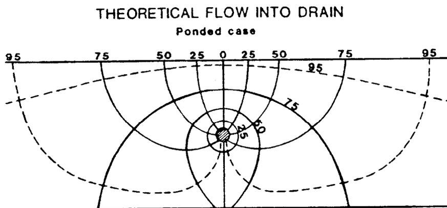
Figure 8. Theoretical flow into a drain.
