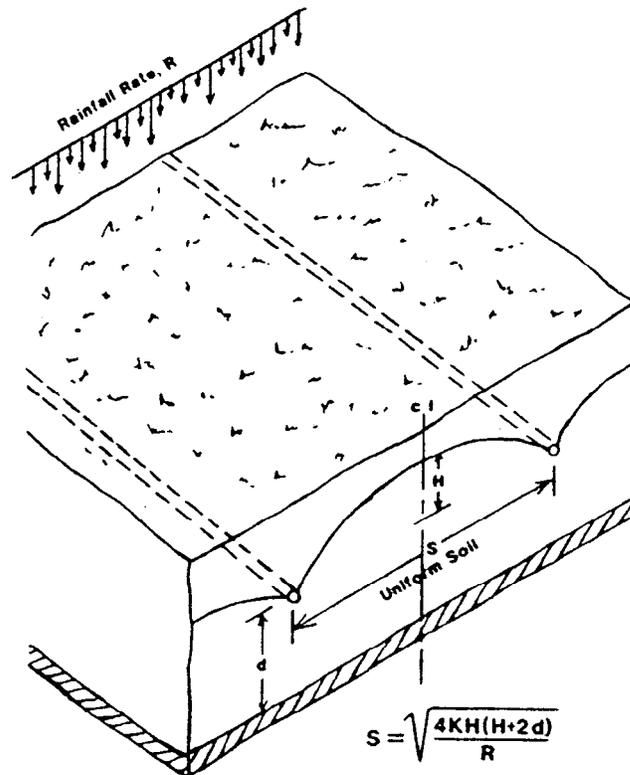
Figure 9. Steady-state drainage condition.
