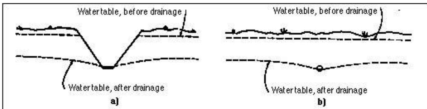
Figure 1. Water table level before and after drainage improvement: a) surface drainage ditch; b) subsurface drainage pipe. (adapted from USDA-ERS, 1987)
