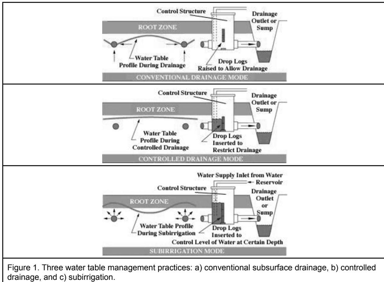
Figure 1. Three water table management practices: a) conventional subsurface drainage, b) controlled drainage, and c) subirrigation.
