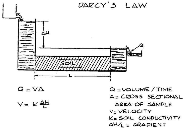
Figure 6. Experiment for hydraulic conductivity measurement.
